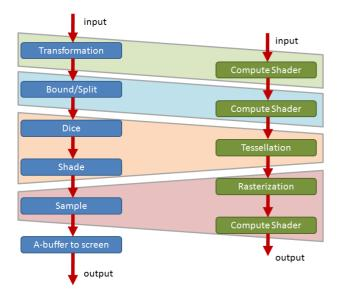
The scheme above shows how REYES pipeline can be mapped on DirectX11 pipeline. Subdivision stage requires recursion – it
